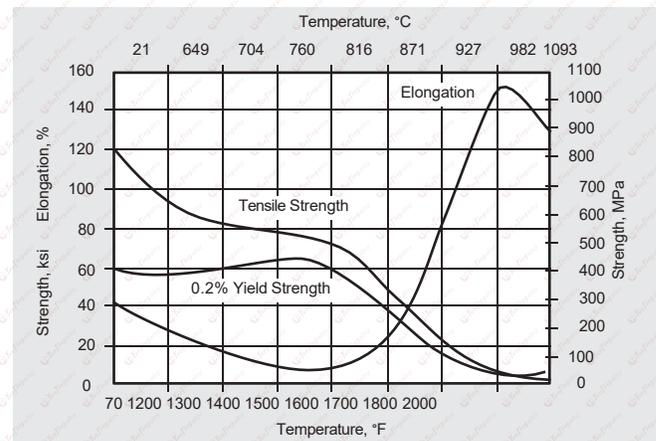
Figure 1. Elevated temperature tensile properties of annealed bar.
